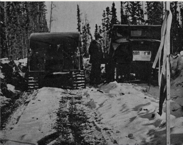
Tracked vehicles are the only ones that can work safely in the muskeg. Even these sometimes sink out of sight
