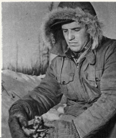
A seismologist plants an electric "ear" that picks up the blast shock waves.
